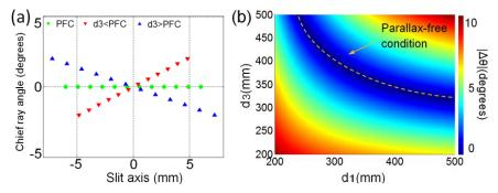
Figure 2. (a). Chief ray angle variations for each lenslet along the slit. Green dots shows PFC, red and blue markers shows two cases where the PFC does not hold. The slit length is 15mm. (b) Choosing f1=20mm, f2=150mm, f3=100mm, and lenslet diameter D=20mm, d2=0, the variation between adjacent chief ray angles is shown in degrees (d4 is forced by the imaging condition-not shown).
