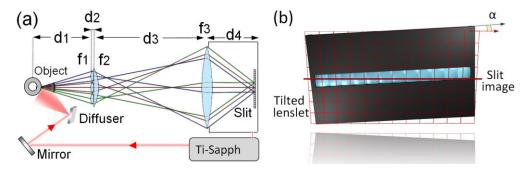
Figure 1. (a) Schematic of the single shot setup. The object is illuminated with diffused 50 fs pulses at 795 nm wavelength and 80MHz rep. rate that are generated with a Ti-Sapphire laser (Ave. power  $\approx$  800mW). The streak camera and the laser are synchronized. (b) 3D model of lenslet tilted around the optical axis. Each lenslet has the diameter of D=3.4mm.
